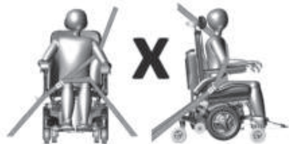
Figure 5.6 - incorrect positioning of three-point occupant restraint
